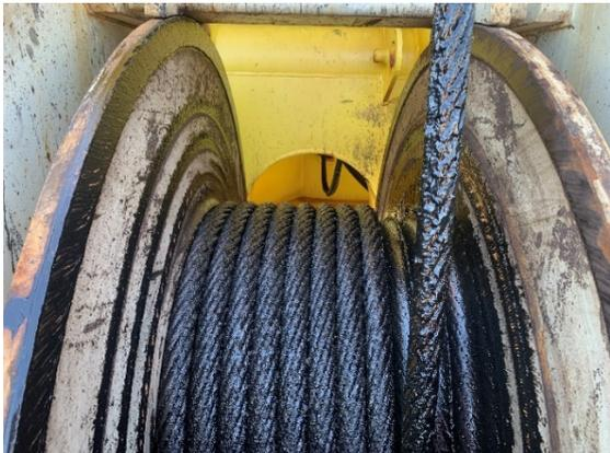
*Luffing hoist drum mild corrosion observed*
