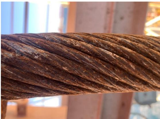
*Main hoist wire rope corrosion observed (near to termination)*
