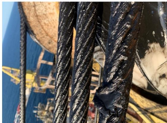
*Luffing wire rope - thick dark grease condition observed*
